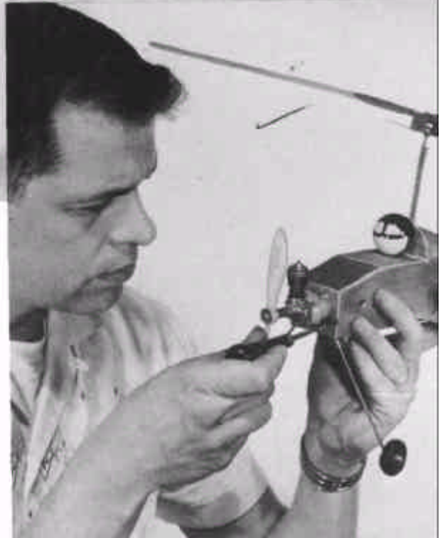
Mount engine on the firewall with four small bolts, using washers under left mounting to provide offset
