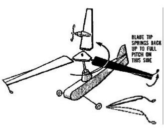
5Blades spring back up on left side to take full bite of air. Since lift is less on rearward stroke away from the wind, the full-pitched blades now balance reduced-pitch blades on opposite side, and the copter flies level.
