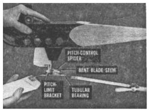
**Underside of rotor hub** shows how spider forces two non-powered blades to tilt at the same angle as powered blade. Wire blade stems are bent at right angles to engage holes in spider plate. Solder parts with hub held flat, upside down, to insure uniform alignment of the blades.
