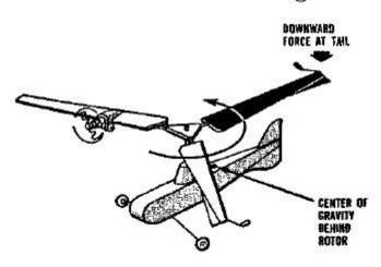
2 To keep a copter level, rotor blades must decrease pitch on forward stroke to balance reduced lift of rearward stroke—called "cyclic pitch." This is done by weighting the model tail-heavy so it pulls down on the blades at the rear—like pushing on rim of a gyroscope.
