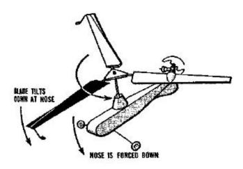
4Blade tips, again acting as a gyroscope, react 90 degrees later to force of air on the right side by tilting down in front. This tips the nose down so the copter, while tailheavy, tilts forward for straight-ahead flight.
