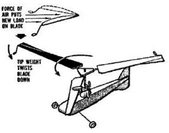
3 Whirling blade-tip weights react 90 degrees later to the force at the tail by twisting blades down on copter's right side. This reduces lift as blades advance into the wind. At same time, air pressure against the downtilted blades exerts a new force on the rotor.
