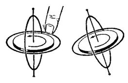
Poke at the rim of a spinning gyroscope and it immediately tilts. But not where you touch it—instead at point 90 degrees past where you touch it. Scientists call this "precession." In the PS helicopter, the whirling rotor acts like a horizontal gyroscope and the propeller blade a vertical gyroscope.
