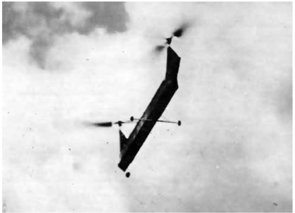
Tandem rubber job. Rotors are Young fly-bar type; Power transmitted through bevel gears at each end of long motor which equalizes thrust. Brake on one rotor permits forward flight.
